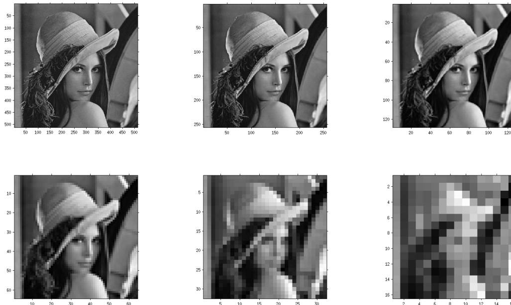
Figure 3: Effect on image quality of reducing the spatial resolution of the image, i.e., the number of samples (pixels) used to represent the underlying continuous intensity signal.
