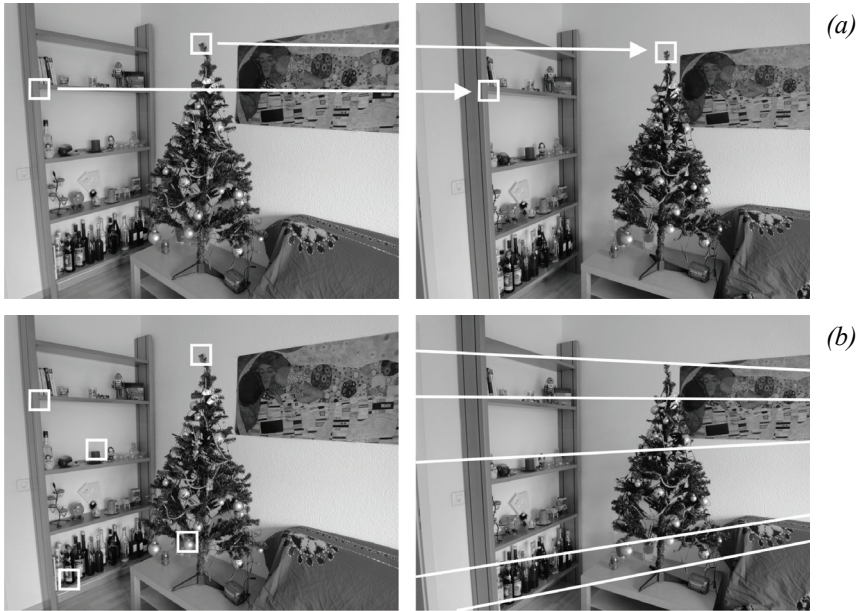
Figure 4.45 A stereo pair. Corresponding points are projections of the same scene point. Because of the epipolar constraint, conjugate points can be searched along the epipolar lines. This heavily reduces the computational cost of the correspondence search: from a two-dimensional search it becomes a one-dimensional search problem.
