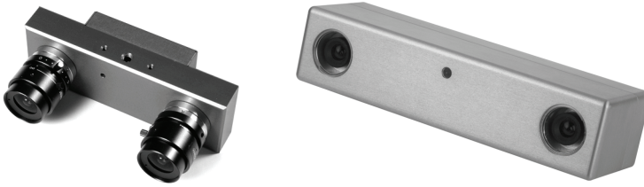
Figure 4.42 (Left) The STH-MDCS3 from Videre Design uses CMOS sensors, a baseline of 9 cm, an image resolution of 1280 \times 960 at 7.5 frames per second (fps), or 640 \times 480 at 30 fps. (Right) The Bumblebee2 from Point Grey uses CCD sensors, a baseline of 12 cm, an image resolution of 1024 \times 768 at 20 frames per second (fps), or 640 \times 480 at 48 fps.
