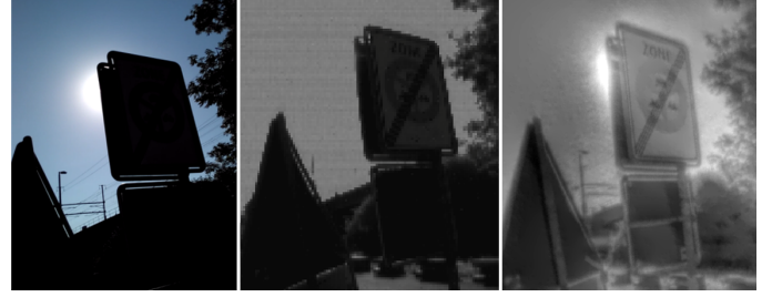
Figure 8. Image reconstruction example. Camera pointing at the Sun, in front of a traffic sign. Left: view from a standard camera, showing severe under-exposure on the foreground. Middle: frame from the DAVIS [4], showing severe under- and over-exposed areas. Right: HDR image reconstructed from the events. Image courtesy of [48].
