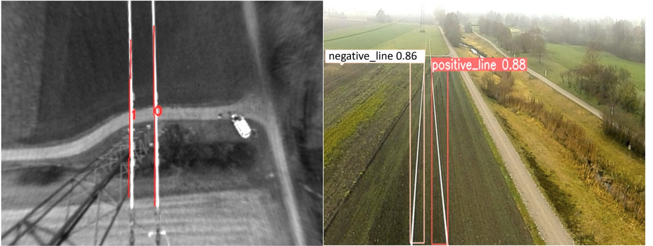
Figure 6: Left) output of the event-based tracker [33]. The algorithm assigns to each tracked line a unique ID. Right) output of the RGB-based tracker [12]. The algorithm assigns to each tracked line its inclination (positive or negative), a confidence score, and a unique ID (not visualized).
