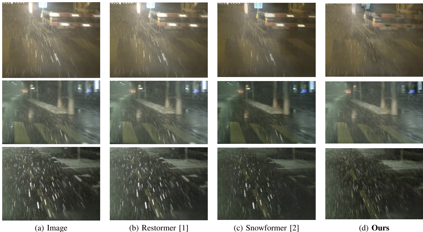
Fig. 12: Qualitative comparison on real driving scenes. (a) Input images, (b)-(c) image restoration baselines, and (d) our results. This shows a magnified region with dense snow and reflective surfaces, highlighting the ability of our method to reduce snow occlusion and preserve scene details under adverse snowfall conditions.
