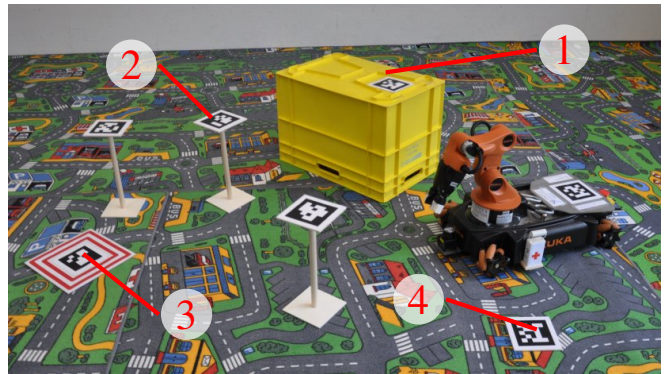
Fig. 4: Mock-up disaster site elements: fixed obstacle (1), movable obstacle (2), goal (3), and origin tag (4).
