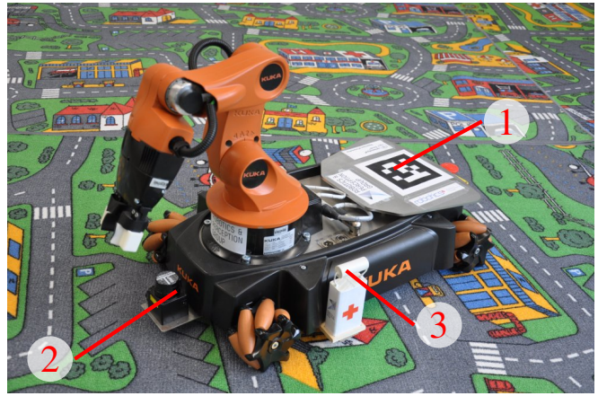
Fig. 3: KUKA youBot equipped with an AprilTag (1), a laser scanner (2), and a first-aid kit (3).
