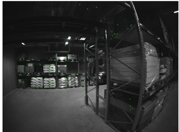
Fig. 5. (a) Features tracked in 'Basement 4' using the LiDAR-based SLAM algorithm A-LOAM. (b) the local environment during a low LiDAR feature event (time approx. 336 s). Close walls and structures reduce the LiDAR measurements, whereas vision based algorithms can still operate normally (the feature tracks of SVO2 [26] are shown).
