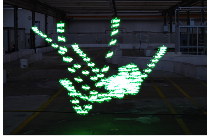
Fig. 6: Feature-based control experiment (HITL). Visualization of flight trajectories with randomly initialized drone configurations.
