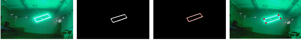
Figure 10: Gate detection pipeline used for extracting gap corners in real-world experiments. From left to right: raw image, segmentation mask after HSV thresholding and noise removal, quadrilateral fitting, and final detected corners (red dots).
