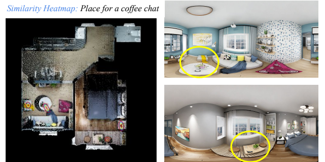
Figure 6. An example of querying an open-vocabulary language query in a GeoSem Map: "Place for a Coffee Chat". On the left, we show the heatmap with GMM covariances and on the right the true locations of the query in the scene.
