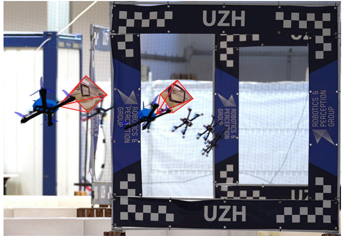
Fig. 1. Real-world deployment of our DreamerV3 policy in the Figure 8 track. During training, the agent learns a world model from interactions with the environment. At the same time, the actor-critic policy is trained by sampling the predictions of the world model, also called imagination . The onboard images consumed by the network are marked in red.
