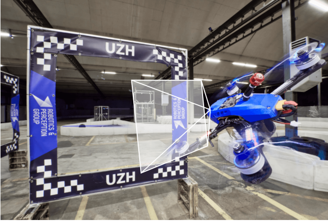
Fig. 6. Real-world experimental setup. Our drone is equipped with a RF receiver similar to that used by professional human pilots. The observations are onboard RGB images, similar to those seen by a human pilot.
