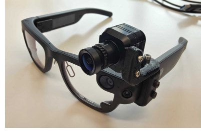
Figure 2. Configuration of the Meta Project Aria glasses with an event camera mounted on top, aligned with the built-in RGB camera to maximize the overlap between their fields of view.
