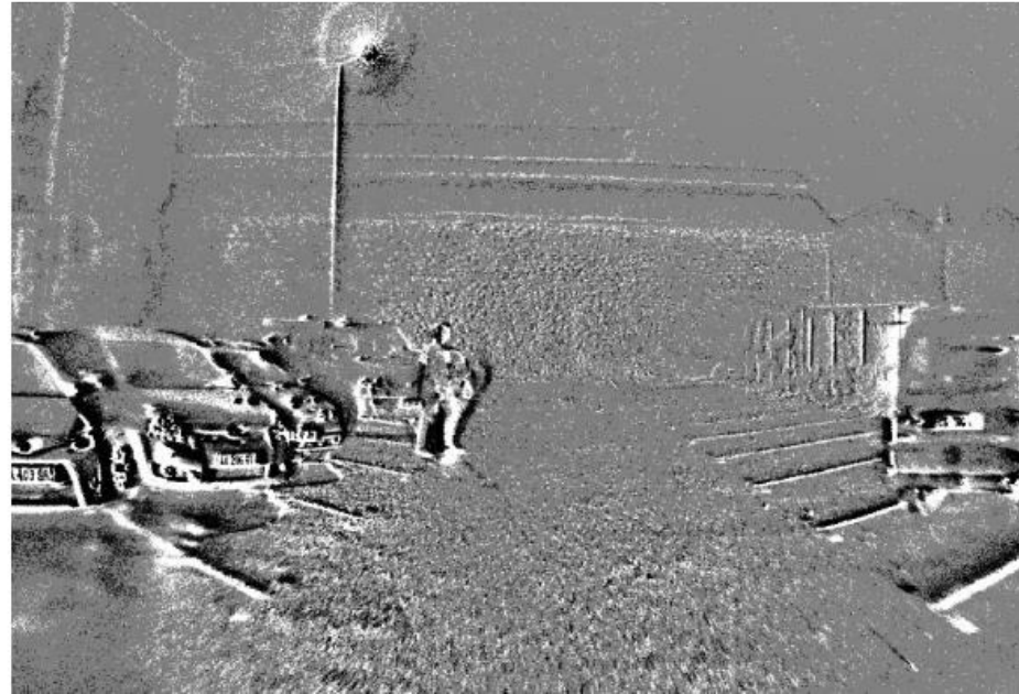
Aggregated event image (pixel intensity equal to the sum of positive (+1) and negative (-1) events in a given time interval)
