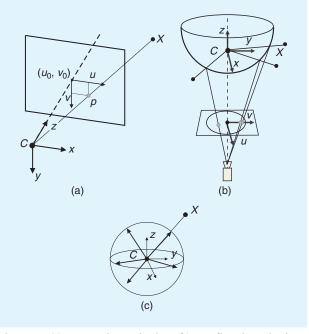
**Figure 3.** (a) Perspective projection, (b) catadioptric projection, and (c) a spherical model for perspective and omnidirectional cameras. Image points are represented as directions to the viewed points normalized on the unit sphere.
