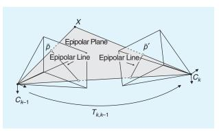
Figure 4. An illustration of the epipolar constraint.
