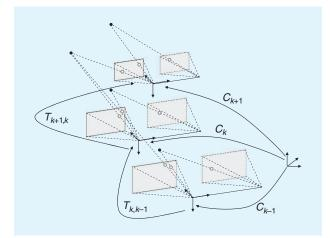
**Figure 1.** An illustration of the visual odometry problem. The relative poses  $T_{k,k-1}$  of adjacent camera positions (or positions of a camera system) are computed from visual features and concatenated to get the absolute poses  $C_k$  with respect to the initial coordinate frame at k=0.
