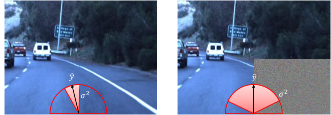
Fig. 1. Uncertainty estimation is necessary to build a safe autonomous driving system. Indeed, a system can be fully functional on a clean image (left), but can return erroneous prediction when processing a corrupted input (right). Uncertainty estimation provides an automatic detection mechanism of such failure cases. The red slices represent one standard deviation from the mean prediction.
