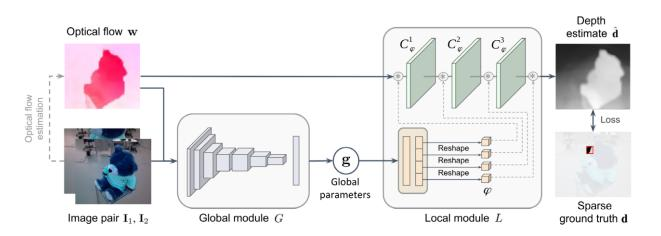
Fig. 2. Global-local model architecture. An image pair and an estimated flow field are first fed through the global module that estimates the "global parameters" vector g, representing the camera motion. From these global parameters, the local module generates three convolutional filter banks and applies them to the optical flow field. The output of the local module is then processed by a convolution to generate the final depth estimate.
