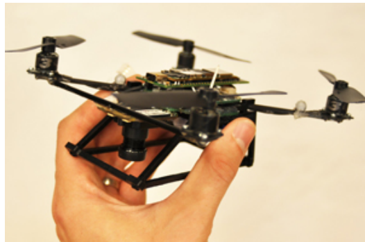
Fig. 1: Our nano quadrotor from KMeI Robotics: a 150g and 18cm sized platform equipped with an integrated Gumstix Overo board and MatrixVision VGA camera.
